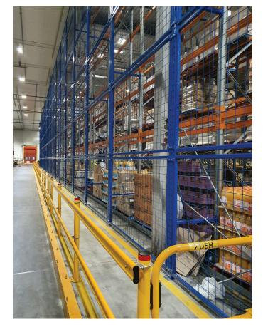
A Safety Mesh Fence is a heavy duty barrier fitted to the rear of single sided pallet racking and is compulsory where pedestrian access is located.
